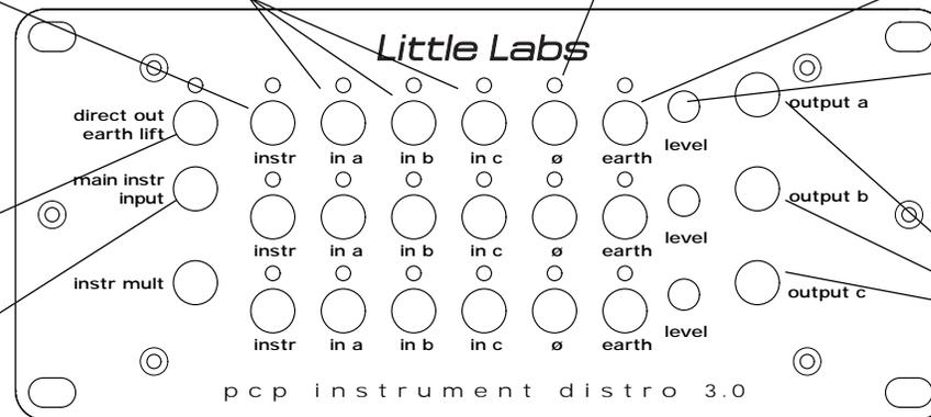
Female XLR inputs to be driven from preferably pro level balanced sources such as a console send or tape machine outputs.
