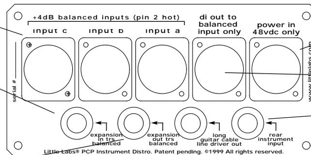
Use only the 48vdc 250ma power supply supplied with the PCP and plug in its 4 pin XLR here.
