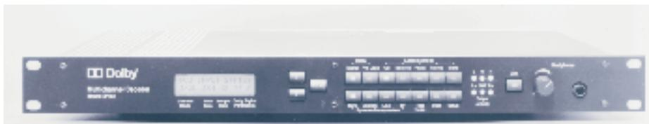
The Dolby DP562 is a reference decoder enabling production, mastering, and broadcast facilities to monitor audio, video, and multimedia programs with multichannel sound. With features tailored to the needs of the professional user, the DP562 is an essential production tool for both Dolby Surround formats and those with Dolby Digital audio, such as DVD and DTV.
