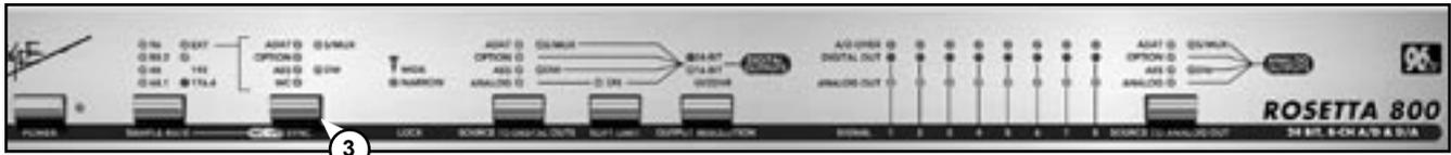
**3) SYNC** – When SAMPLE RATE is set to *EXT*, the SYNC parameter determines the source of the unit’s clock.
